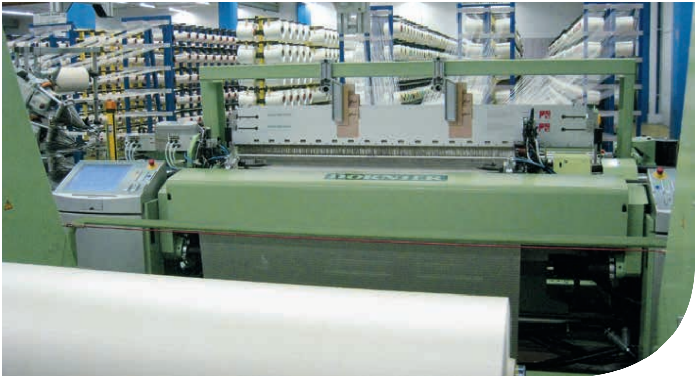
A1 air-jet weaving machine for tire cord
